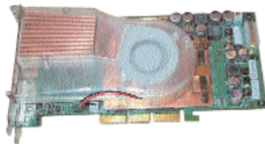
The enormous air intake duct and heat pipe solution help keep the GeForce FX cool
